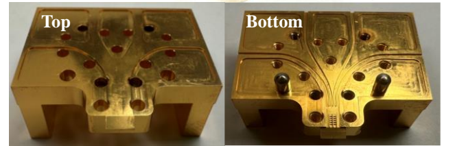
Fig. 5. Photographs of the prototype antenna fabricated by CNC milling.
