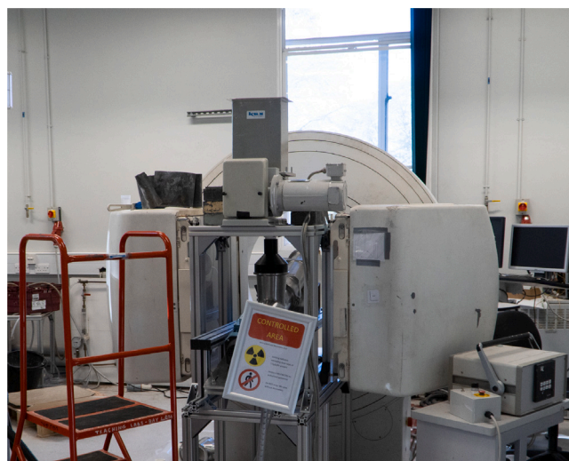
Fig. 1. Picture of the Experimental Set-up; supporting frame holding the blender and feeder in the ADAC detector’s FoV.
