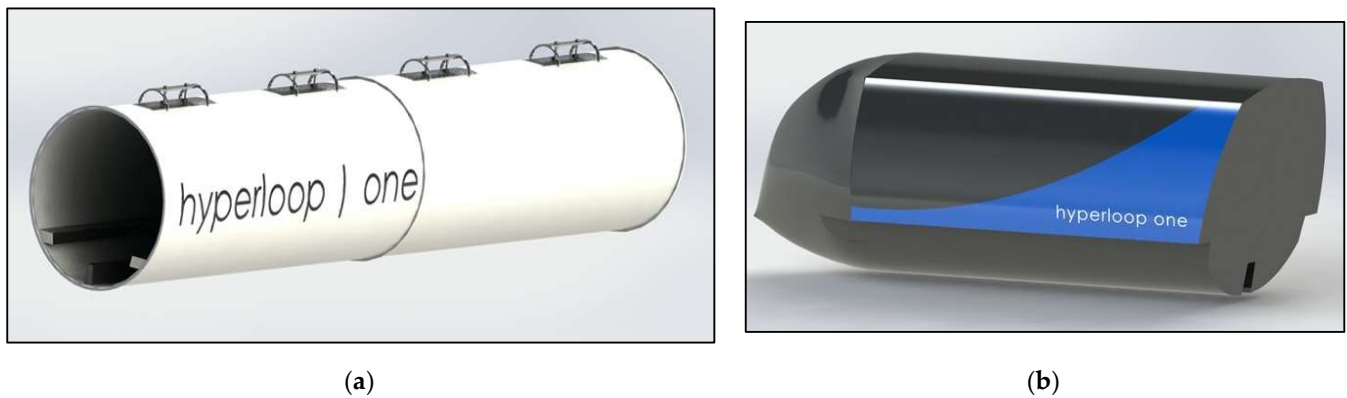
Figure 3. (a) 1:1 Solidworks design of Virgin Hyperloop One test track (b) Virgin Hyperloop XP-1 Pod. Both models are to be imported into LS-DYNA as a STEP file for blast loading simulations.
