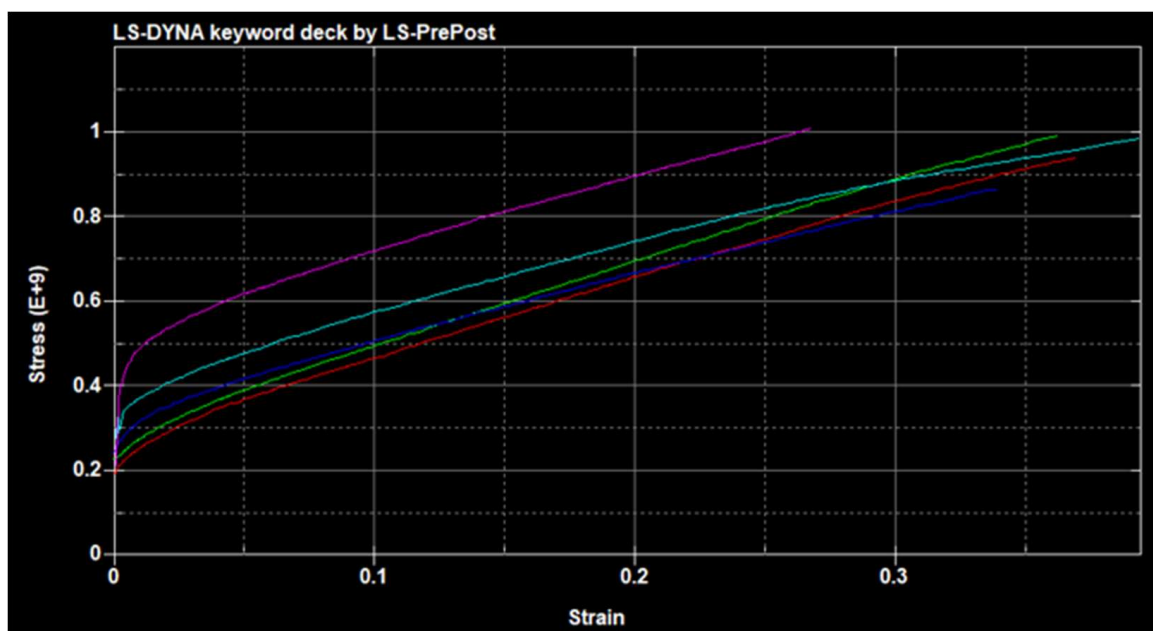
Figure A1. LS-DYNA Material graph showing stress/strain characteristics of steel at varied loading levels (Stress in Paskal): red: low strain rate; green and blue: moderate strain rate; and purple: high strain rate.
