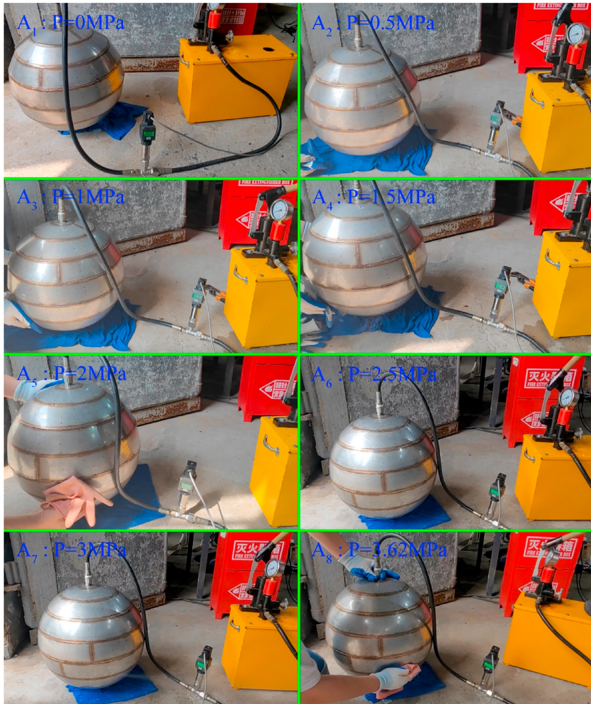
Fig. 11. Dieless bulging of the longan-shaped pressure hull under various internal loads.
