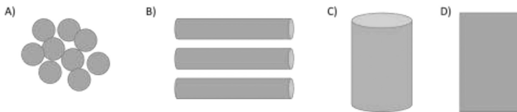
Fig. 34. Different geometries for EPCMs (a) spherical (b) tubular (c) cylindrical and (d) rectangular [153].
