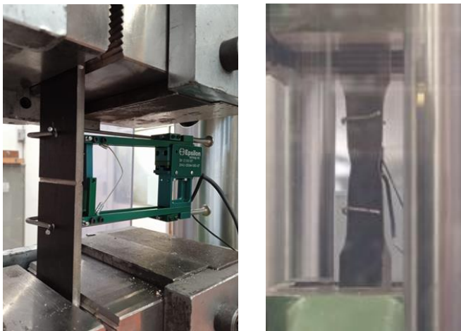
Figure 3 A tested notched specimen with the extensometer attached at the ends of the gauge length (left), observation of the necking in the reduced area of an unnotched specimen during testing (right).
