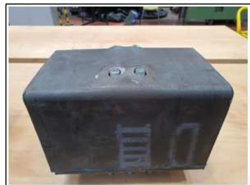
Figure 9: Hollow-section wall deformation of the FFT specimen
