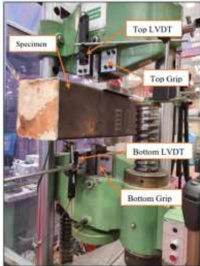
Figure 3: The experimental setup
