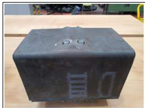
Figure 9: Hollow-section wall deformation of the FFT specimen
