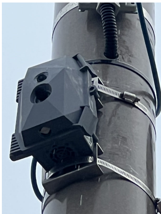
Figure 1. An image of Traffic Ear mounted on a street column in the metropolitan borough of Sandwell, West Midlands, UK.
