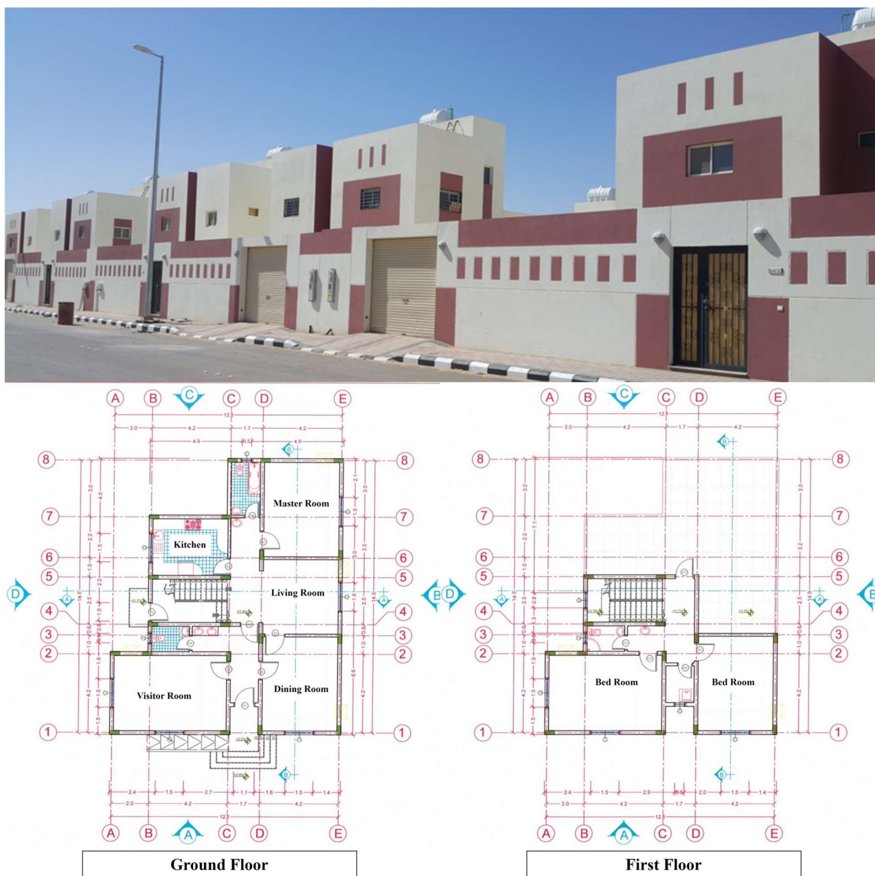
Figure 13. The design of the residential units' ground floor, first-floor plane, and perspective.
