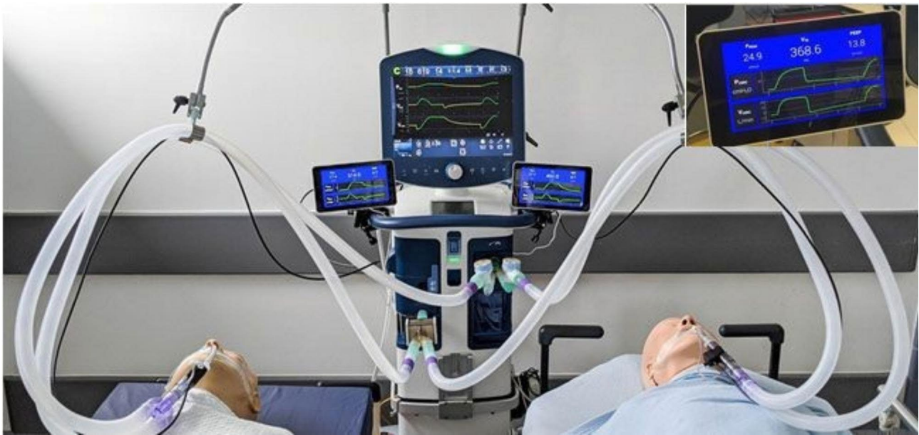
Fig. 2 VentShare System attached to two manikins. Monitoring of the respiratory parameters for each limb are shown to the right and left of the main ventilator. A closeup of the display readout is also shown
