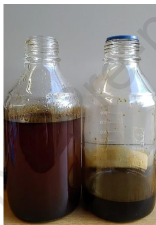
Figure 6 Aqueous phase (on the left) and pyrolysis oil (on the right) of Solid Grade Laminate
