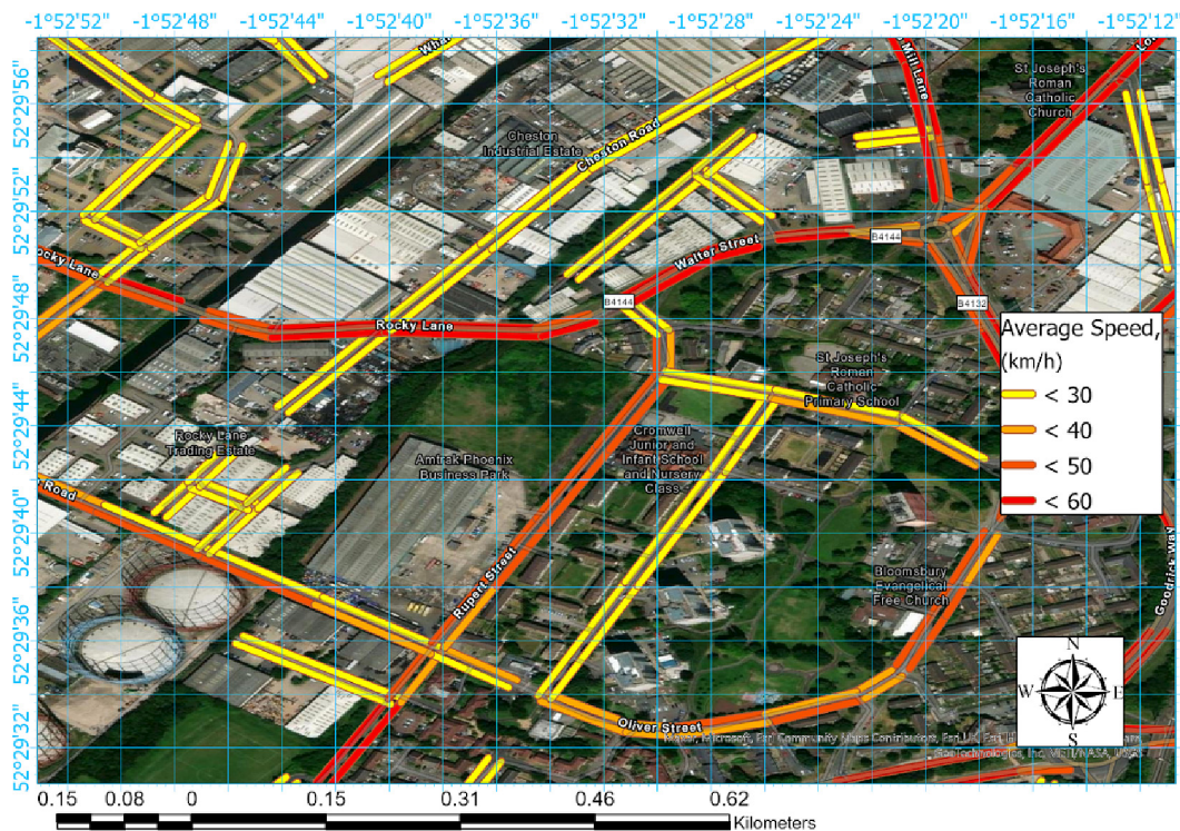
Fig. 1. GeoST mapping of urban mobility over streets in the Ladywood area of the city of Birmingham within the West Midlands in the UK; the average speed (km/h) over 07:00–09:00 Mondays 2018.
