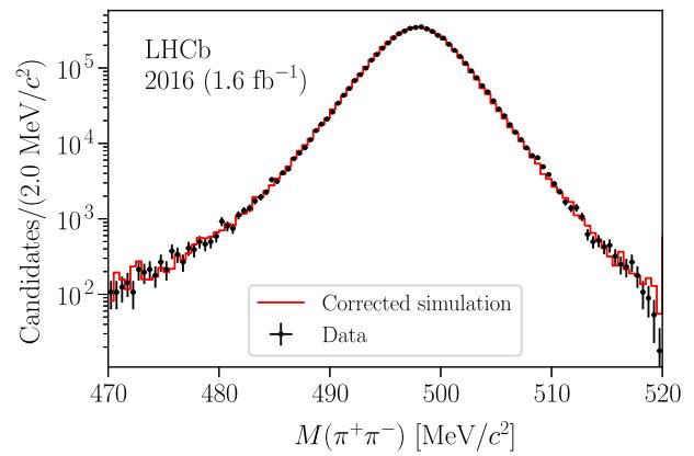
FIG. 2. Invariant-mass distribution of  $K_S^0 \rightarrow \pi^+ \pi^-$  candidates in 2016 trigger-unbiased data (points with error bars) and corrected simulation (solid histogram). The histogram of simulated candidates is normalized to data.
