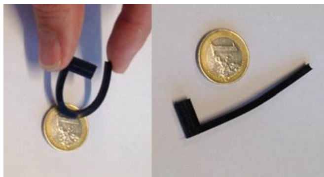
Fig. 27. 3D printed flexible antenna enabled by LM [178].
