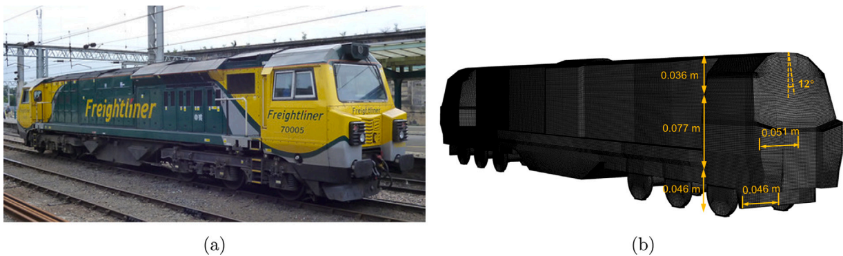
Fig. 27. The Class 70 validation case locomotive. (a) Class 70 locomotive (b) the CFD mesh and key dimensions, given here in the reduced 1/25th scale in m.
