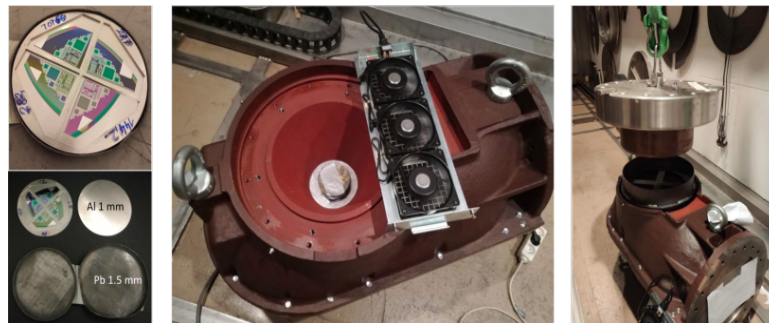
Figure 3. The sample holder for the ^{60}\text{Co} irradiation at UJP Praha, made with material thickness of 1.5 mm Pb and 1 mm Al to minimise the dose induced from scattered low energy charged particles and to achieve Charge Particle Equilibrium according to Total Ionising Dose Irradiation Standards [4].
