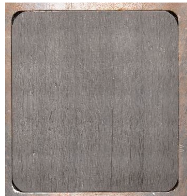
Figure 4. Front surface of the UHTCMC material.
