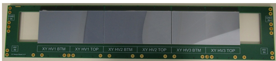
Figure 8. First attempt at assembling an XY sensor board with three tiled XY sensors.
