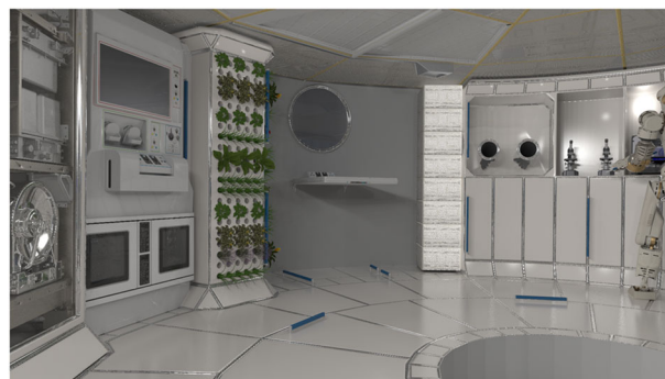
Fig. 2 Supporting habitation and research in deep-space. A module within a deep-space habitat, containing a plant growth wall, essential for conversion of carbon dioxide to oxygen, robotic assistance, scientific kit (microscopes) and a glovebox to allow the contained manipulation of objects. Image credit: NASA 36 .
