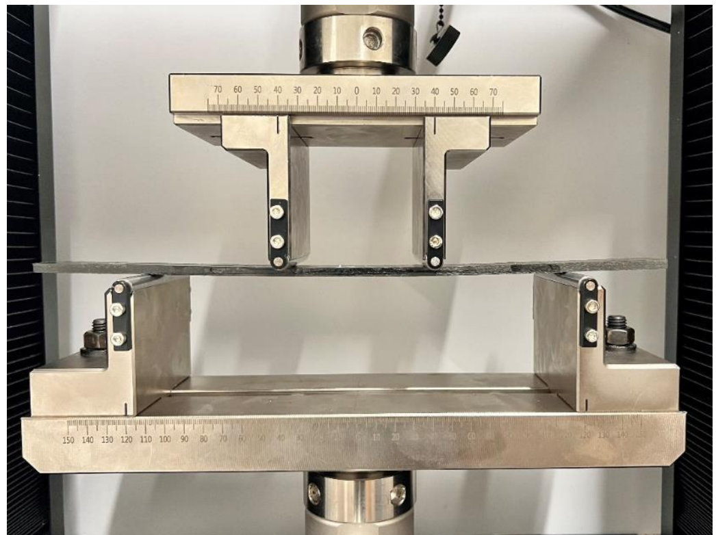
Figure 3. Repaired specimen under four-point bending test.
