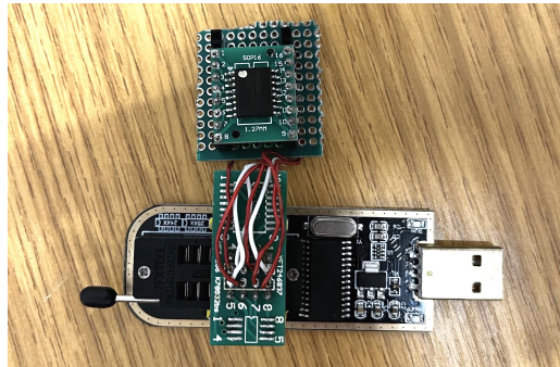
Figure 3: Dumping BMC firmware with a flash programmer.
