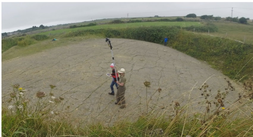
Fig. 2. Demonstration of the image capture system in action, used to take photos of the quarry surface for the 3D model by undergraduate researchers Harry Jones and Lewis Haller in August 2021 at Spyway Quarry. Photograph taken on a GoPro HERO3+ Silver Edition camera positioned above an exposed vertical quarry face in the east of the quarry.
