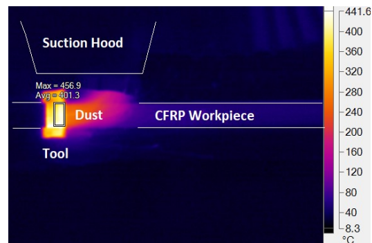
Figure 6- Infrared thermogram captured during the trimming operation.
