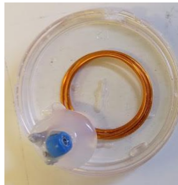
Figure 4. Circular repeater coil.
