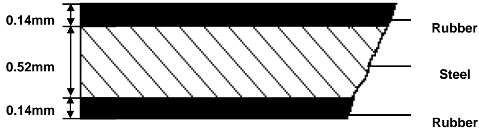
Figure 6, Schematic of three layer shim design
