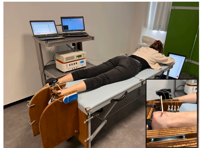
Fig. 1. Image of the experimental setup. The participant was positioned in prone with the foot secured within a dynamometer with the ankle in 0° of dorsiflexion/plantarflexion. Force feedback was presented to the participants in real time. The bottom right box shows a detailed image of the tapping device and accelerometers.
