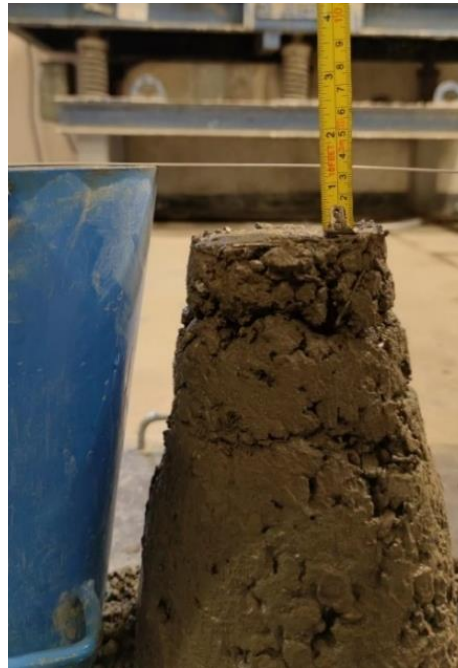
Figure 1. Slump test of the M_3 concrete mix.
