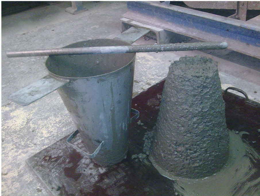
Fig. 2: Typical slumped test
