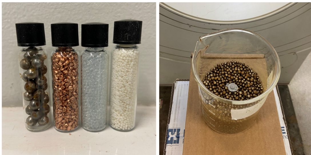
Fig. 4. A small sample of four of the materials used to induce attenuation (left). From left to right: steel, copper, glass, and MCC. The beaker is filled with steel balls and the source is placed in the centre of the field-of-view (FOV) of the Forte (right).
