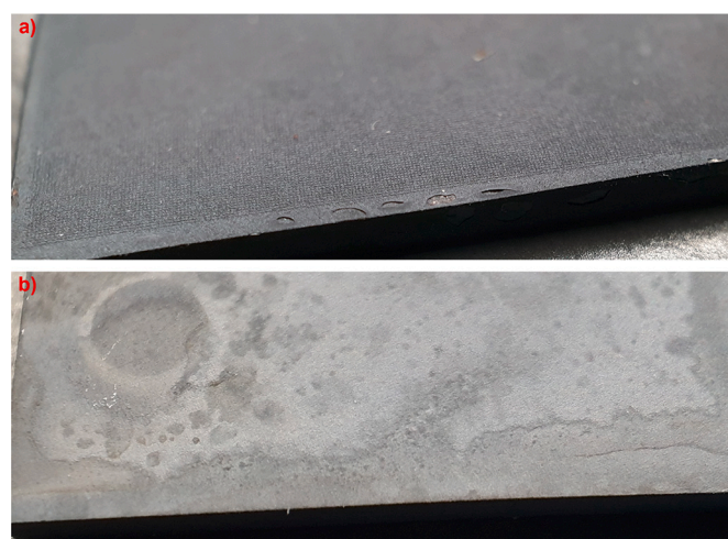
Fig. 7. Optical images of a) laser-treated and b) non-treated SS310 samples after the corrosion experiment.
