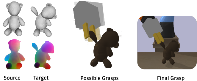
Fig. 1. Deformable object grasping by the proposed grasp transfer method. (left) Source and target meshes, and their functional maps. (middle) Transferred possible grasp configurations. (right) Executed best grasp.
