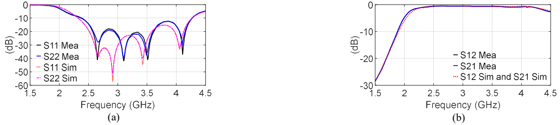
Fig. 7. The measured and simulated S-parameters of the SIW with no liquid metal i.e. with wall in OFF state. (a) reflection coefficients ( S_{11} and S_{22} ) and (b) transmission coefficient ( S_{21} and S_{12} ).
