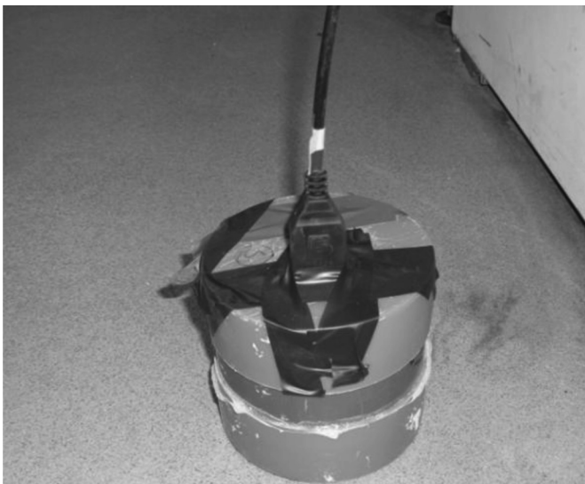
Fig. 2. Completed sample with TDR probe inserted.
