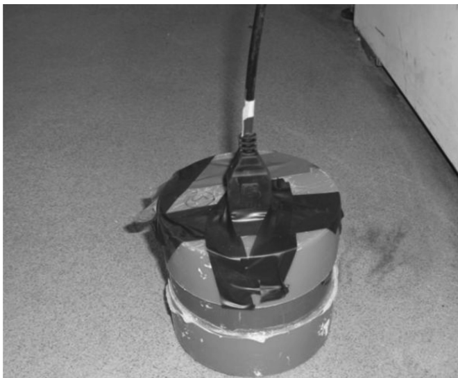
Fig. 2. Completed sample with TDR probe inserted.
