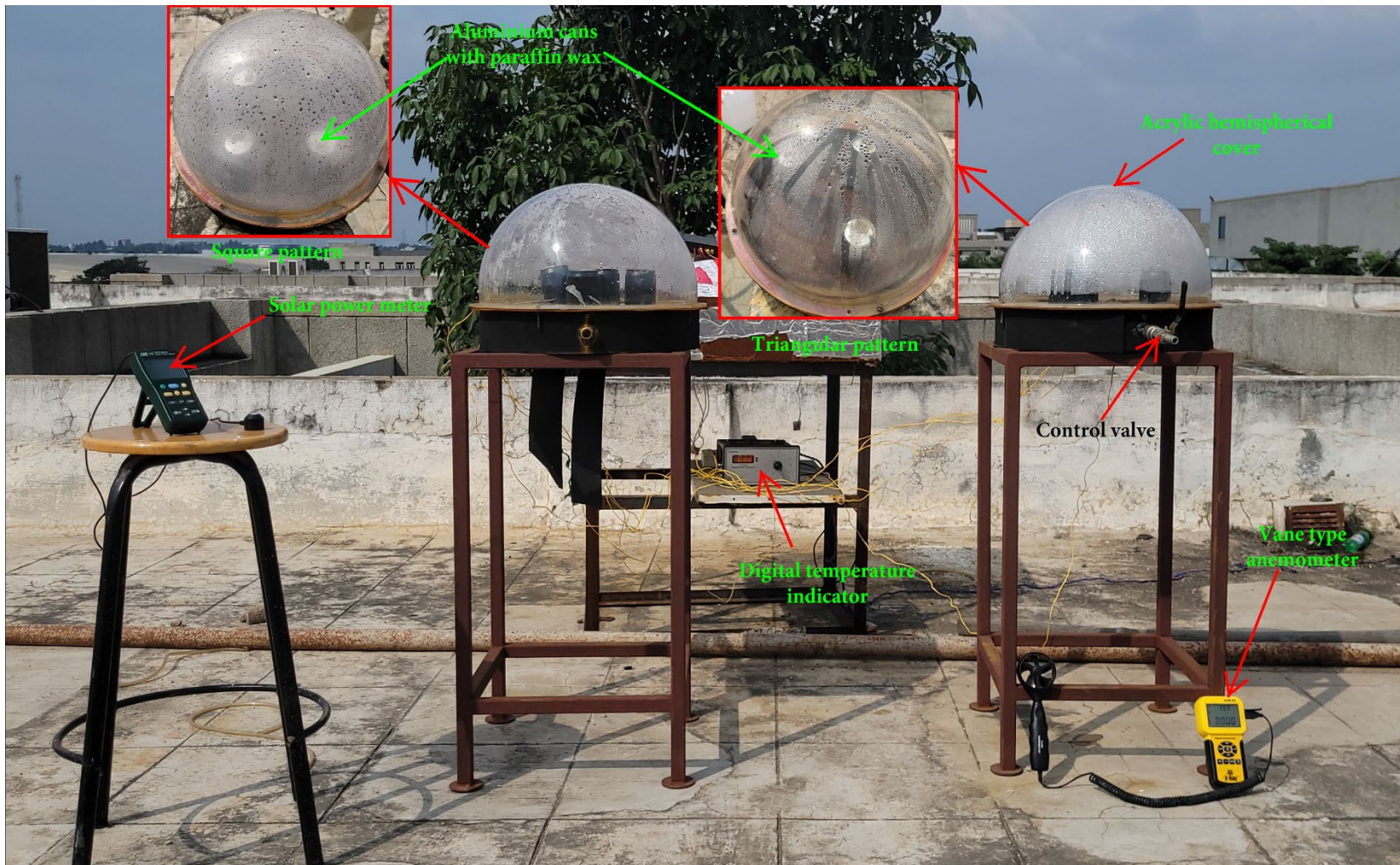
Fig. 2 Photograph of the experimental set-up with cans placed inside the basin
