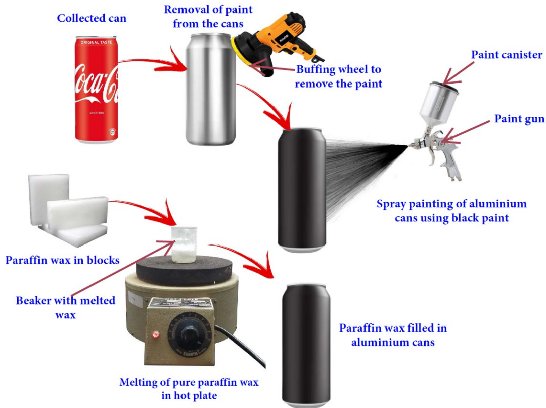
Fig. 3 Steps involved in preparation of paraffin wax encapsulation in cans
