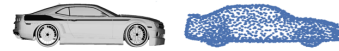
Fig. 1. A digital car represented as 3D polygonal mesh and 3D point cloud.
