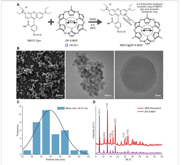
FIGURE 1 (A) Schematic showing the structure of ZIF-8 MOF nanoparticles and interaction of RBITC with ZIF-8 MOF nanoparticles. (B) SEM and TEM images of ZIF-8 MOF nanoparticles show the particle size and morphology. (C) Size distribution of ZIF-8 MOF nanoparticles. (D) X-ray diffraction pattern of ZIF-8 MOF nanoparticles indicates the phase purity of the nanoparticles.
