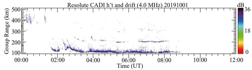
**Figure 3.** Sequence of group range at 4 MHz by Canadian Advanced Digital Ionosonde (CADI) at Resolute Bay station during the interval of interest of 00:00–12:00 UT on 1 October 2019 between the virtual height of 100–500 km.
