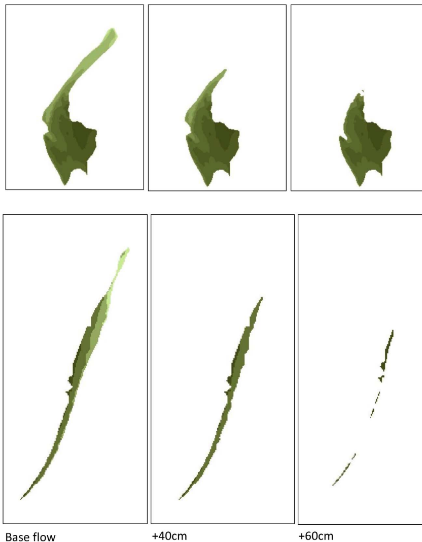
Figure 1. Digital Elevation Models showing the different extent of habitat loss under low, medium and high flows for representative gravel bars with (a) elevated profile and (b) shallow profile. Figure 1a shows patch 10, a large area, complex habitat patch, of which only 28% is submerged when levels are 1 m above base flows; Figure 1b shows patch 15, a low elevation habitat patch, of which 100% is submerged under the same conditions. doi:10.1371/journal.pone.0061866.g001
