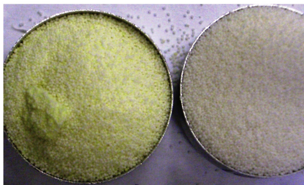
Fig. 2. Gross colour change of MCC samples after RESS-WTS coating.
