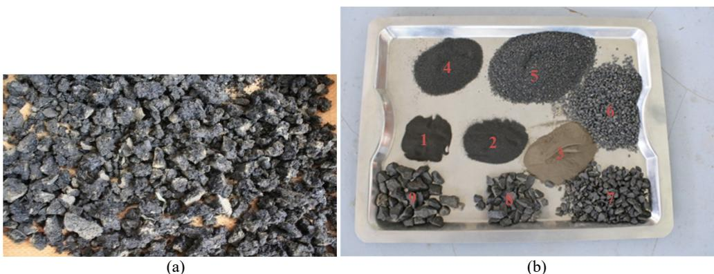
Fig. 5 RAP material: hand crushed (a) and gradation after binder extraction (b) [1 – 75 $\mu$ m, 2 – 150 $\mu$ m, 3 – pan, 4 – 300 $\mu$ m, 5 – 600 $\mu$ m, 5 – 5mm, 6 – 9mm, 7 – 12mm, 8 – 14mm, 9 – 19mm].
