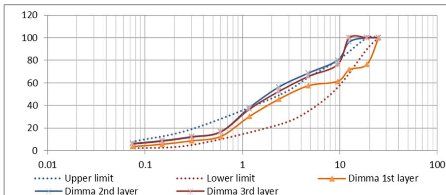
Fig. 7 Aggregate gradation of different layers of same road.
