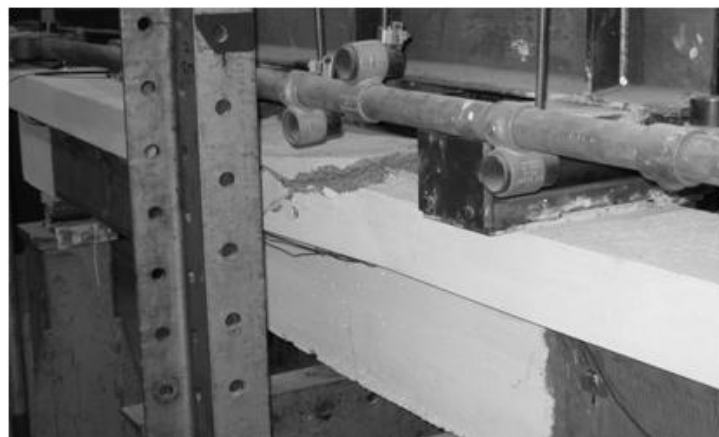
Fig. 8–Flexural failure of F/295/LP1/3.3.
