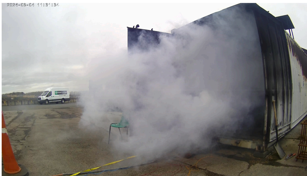
Fig. 3. The white vapour produced following nail penetration of a single automotive module (Envision-AESC module containing 8 x 53Ah NMC pouch cells) [154].
