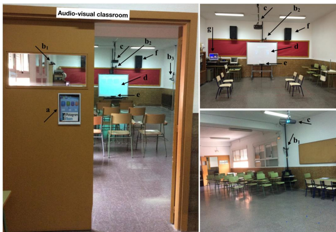
Figure 2. Room arrangement: (a) board for the children to place the PECS symbols, (b 1,2,3 ) video cameras, (c) projector, (d) IDW, (e) Kinect, (f) speakers, and (g) PC screen displaying the video captures. Note. Four chairs were placed in front of the IDW to show the dimensions of the play area but they were not used during playtime. In the study sessions, the PC screen (i.e., (g)) was hidden behind a paper screen so children could not see it and get distracted.
