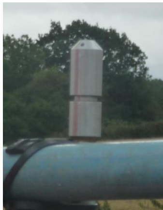
Figure 4 Pressure probes used for pressure transient measurements
