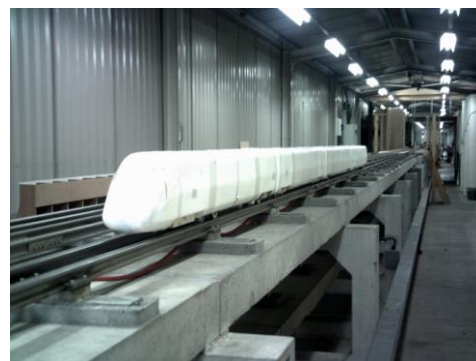
Figure 8 The University of Birmingham moving model (TRAIN) rig
