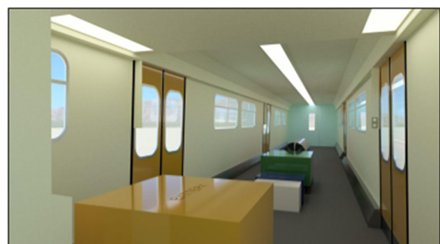
Fig. 2 Early concept render of HydroFLEX hydrogen-hybrid powertrain located within the PMOS carriage. Note that the specific equipment is not modelled yet as configurations were being trialled at this stage. The equipment from the nearest the viewpoint outwards is the battery, DC/DC converter, Ballard fuel cell and representative type 4 hydrogen tank
