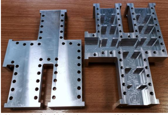
Fig. 21. Photograph of the fabricated resonant manifold triplexer.
