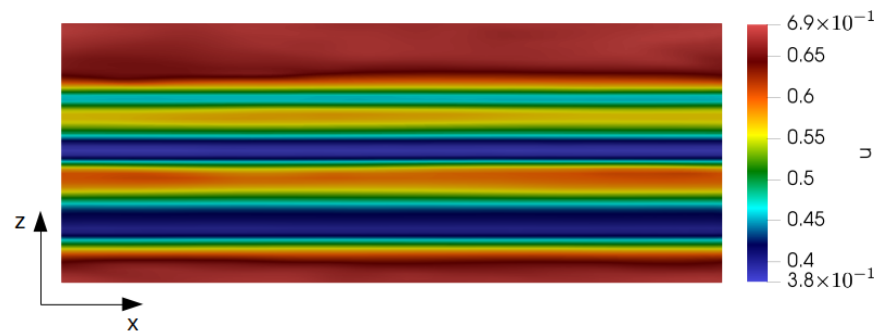
Figure 18. Instantaneous velocity contour in streamwise direction at xz plane—HMF.
