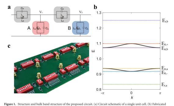
**Figure 1.** Structure and bulk band structure of the proposed circuit. (a) Circuit schematic of a single unit cell. (b) Fabricated sample with 10.5 (21 circuit node) unit cells. (c) Band structure of the bulk circuit with  $r_a = 1.2$ ,  $r_b = 1.8$ ,  $s_a = s_b = 1$ . The dashed lines mark the six critical frequencies of the bulk circuit.
