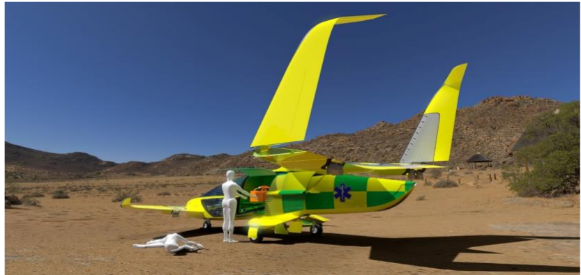
Figure 24. First responder eVTOL concept vehicle. Image courtesy of Dean Mangurenje and Dr. Mike Bromfield, Coventry University, UK
