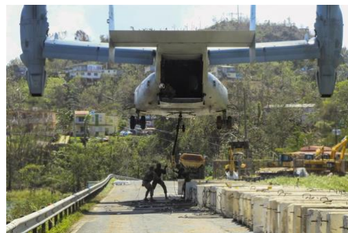
Figure 15. Marines attach a barrier to a V-22 Osprey tilt-rotor aircraft. Image: US Army
