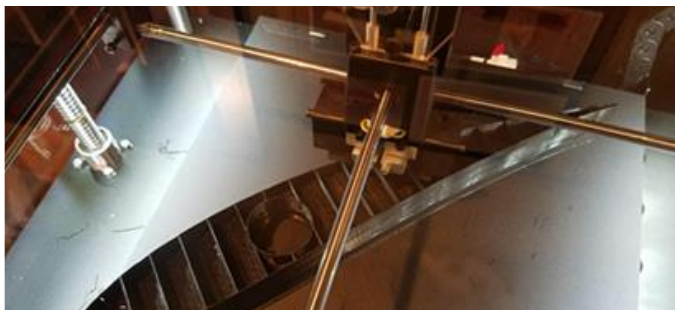
Figure 42. 3D printing of a wing airfoil section assembly with integrated structural elements by International Vehicle Research. Image courtesy of Johnny Doo
