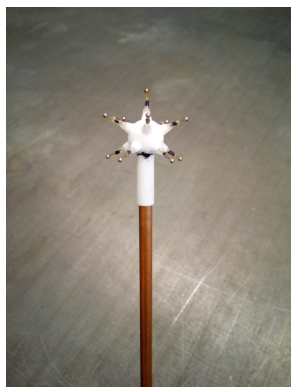
Figure 6. ACHINOS with 11 balls of \varnothing 2 mm constructed using 3D printing [18].
